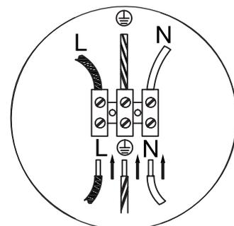
Details of terminal wiring.
